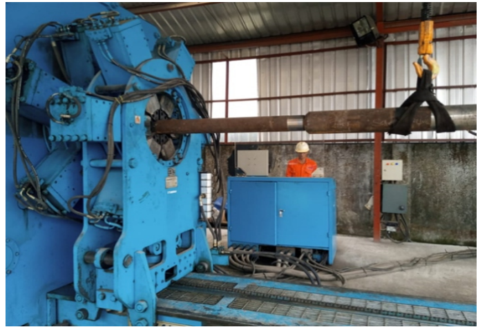
BUCKLING MACHINE THAT CAN BUCK FROM 2-3/8 TO 24" OUTSIDE DIAMETER
